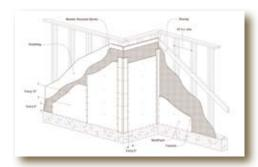
• It is recommended that APA rated 7/16" OSB (Oriented Strand Board) or plywood sheathing be used to ensure nail-holding powera and provide an air gap between board and sheathing.
