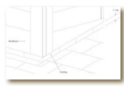
from soil grade or 1" - 2" from hard surface to the starter strip and boards as per local building codes.
