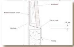
roofing manufacturer's instructions flashing and counter-flashing are required. NichiProducts must be installed with a minimum 1" clearance from roofing as per local building codes.
