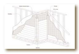
• Trim should be fastened a minimum of 3/4" from trim edges when using screws or 1/2" from trim edges when using finishing nails, and spaced a minimum of 16".
